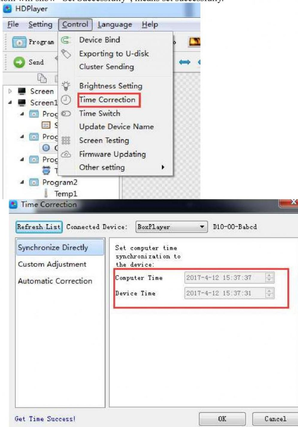
Fig.6-5 Synchronous Correction
